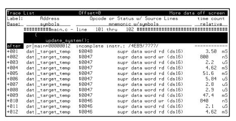
Notice the trigger state (line 0, labeled "after") is included in the trace list; trigger states are always stored.
