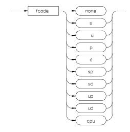
The function code is used to define the address space being referenced. Select the appropriate function code from those listed below.
